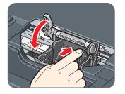
6 Make sure that the Print Head is installed properly.
