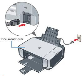
N Important • Plug the power cord all the way in, since it may be difficult to plug.Make sure that the Document Cover is closed. • Do NOT connect the USB cable at this stage.
