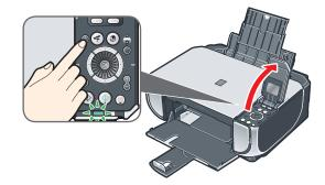
4 Use the  $\blacktriangle$  or  $\checkmark$  button on the Operation Panel to select the language for the LCD, then press the **OK** button.
