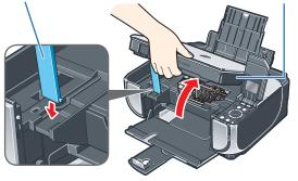
**6** Write down the serial number located inside the machine. You will need this to register your product.
