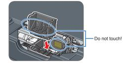
**5** Push the Print Head to hold it in place, and lower the Print Head Lock Lever carefully.
