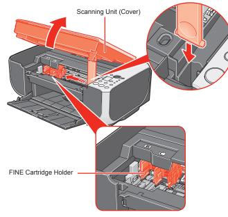
Do not touch internal parts other than the FINE Cartridge Holder.
