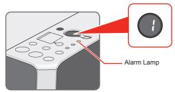
If the **Alarm** lamp lights and an error code is displayed on the LED, refer to "An Error Code Is Displayed on the LED" in "Troubleshooting" of the Quick Start Guide.
