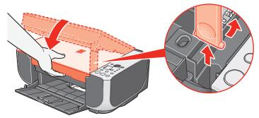
Once you have installed the FINE Cartridges, the LED will flash green. Wait until the LED stops flashing and displays 1. It takes about one to two minutes
