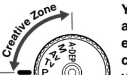
You can set the shutter speed and/or aperture and change the exposure as desired. By changing the camera settings, you can obtain various effects.
