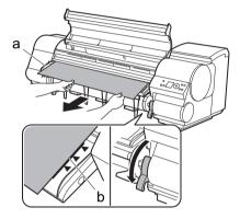
• Do not force the roll paper into alignment with the **Paper Alignment Line** (b). This may prevent the paper from being advanced straight.
