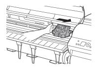
• Always move the **Carriage** to the right side. If the **Carriage** is on the left, a **Carriage** error may occur when you turn on the printer.
