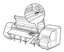
• If the **Cutter** is on the left side, be sure to move it to the right. If the **Cutter** is on the left side when you turn the printer on, the printer may rip the paper.
