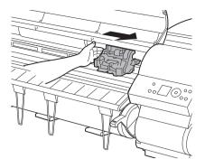
• Always move the **Carriage** to the right side. If the **Carriage** is on the left, a **Carriage** error may occur when you turn on the printer.
