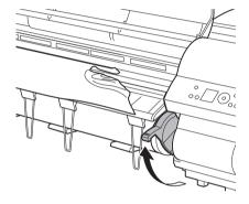
Holding the paper on both sides, pull the jammed portion out toward the front. Use a scissors or cutting tool to cut away the printed or wrinkled portion.
