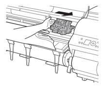
If the **Cutter** is out, move the **Cutter** to the right side, away from the paper.
