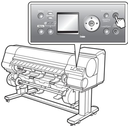
**2** When the following screen is displayed, press **▲** or **▼** to select the language used on the display screen, and then press the **OK** button.
