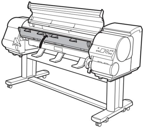
**5** Attach the four **Ejection Supports (a)** on the back of the **Ejection Guide**.
