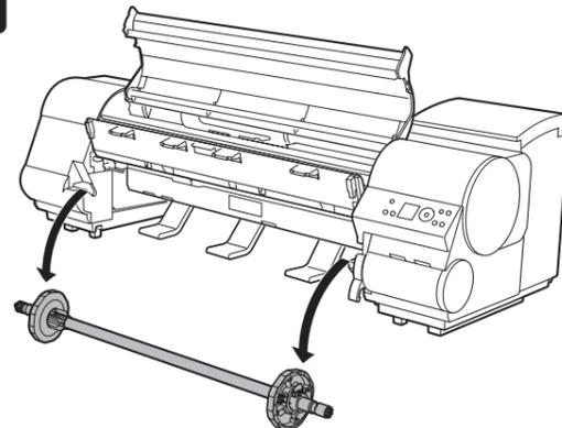
**4** Lift the **Holder Stopper** lever (a) from the shaft side to unlock the stopper. Holding the **Holder Stopper** at the position indicated (b), remove the stopper from the **Roll Holder**.
