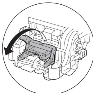
**6** Lift the **Printhead Fixer Cover** to open it fully.
