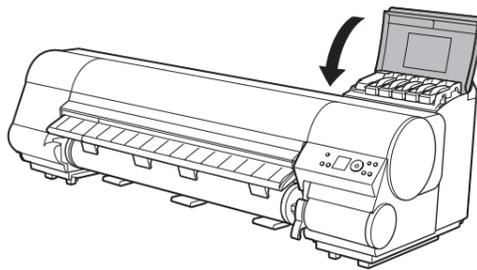
After you have installed the **Printheads** and all **Ink Tanks**, the system is automatically filled with ink for the first time. This process takes about 14 minutes. In the meantime, install the printer driver and manual.
