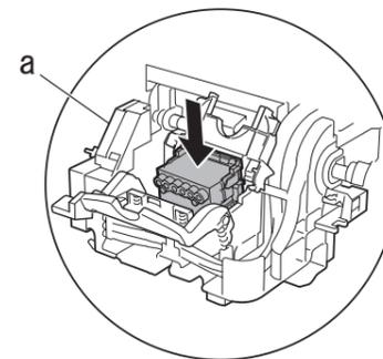
**10** Pull the **Printhead Fixer Cover** down toward the front to lock the **Printhead** in place.
