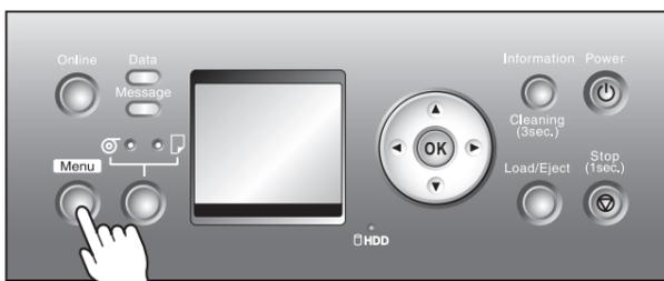
**2** Press **▲** or **▼** to select **Interface Setup**, and then press the **▶** button.
