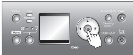
After loading a roll, the printer automatically shows a menu for selection of the paper type on the **Display Screen** and beeps.
