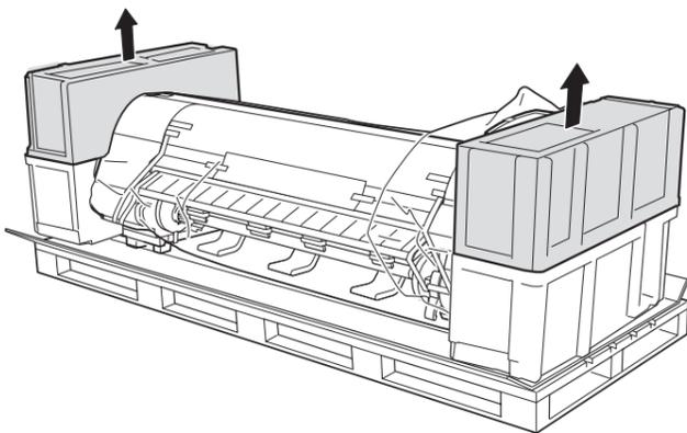
**2** While two people hold the carrying handles under the printer on one end and lift the printer a little, have a third person remove the packaging material and the plastic covering from under the printer. After the packaging material has been removed, lower the printer.
