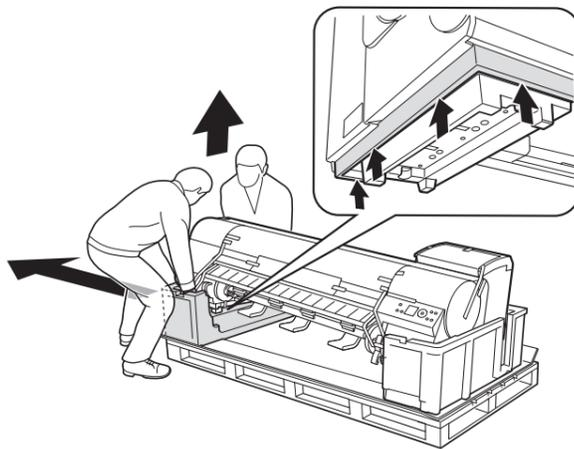
**3** Remove the packaging material and the plastic covering from the other side of the printer the same way.
