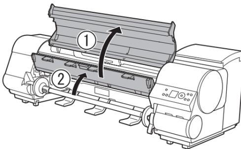
**3** Remove the **Roll Holder** from the printer.
