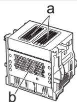
**8** Remove the orange **Safety Cap 1** (a). To remove **Safety Cap 2** (b), push the grip (c) as you remove the cap.
