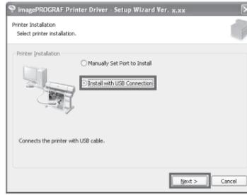
**8** When the following dialog box is displayed, make sure the printer is on and use the USB cable to connect the printer to the computer.
