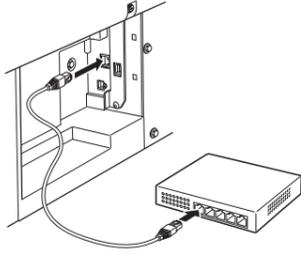
**MEMO** • If the printer is on, the Link indicator is green for 100Base-TX connections and amber for 10Base-T connections.
