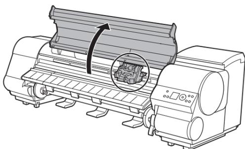
**5** Pull the **Printhead Fixer Lever** forward all the way to open it completely.
