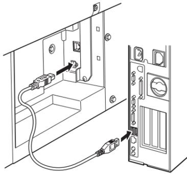
**MEMO** • Be careful not to insert the USB cable into the Ethernet port.
