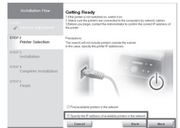
**8** On the **IP Address Specification** window, enter the desired printer's IP address and click **Install** to start the installation process.
