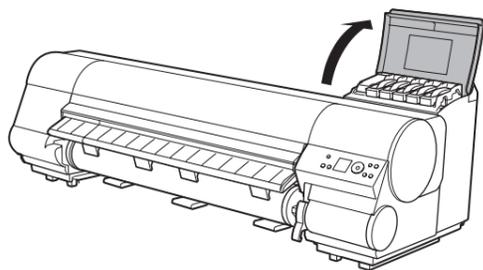
**2** Lift the stopper (a) of the **Ink Tank Lock Lever** of the color to load. Lift the **Ink Tank Lock Lever** until it stops, and push it down to the front.
