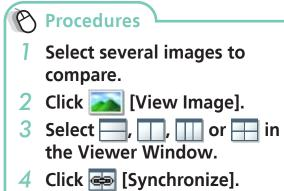
Selecting [Synchronize] causes actions such as increasing/reducing the magnification level or scrolling around the image to apply to all of the selected images in lock step, making it easy to check minute details of focus, coloring and other image characteristics.
