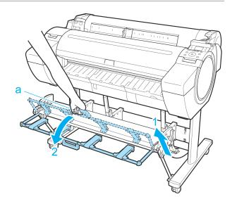
Open the Output Stacker Ejection Guides (a). This completes the procedure of switching to Extended position B.
