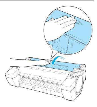
Fold an A4 sheet lengthwise four times and insert it through the gap of the Paper Feed Slot. Push the scrap out toward the Platen.
