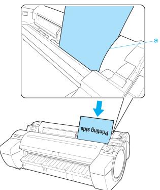
Move the Width Guide (a) carefully to match the size of paper loaded.
