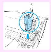
4 Push the lnk Tank Lock Lever closed until it clicks into place.
