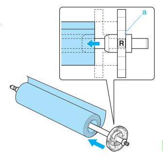
Insert the Holder Stopper from the left in the Roll Holder as shown. Holding it at the position shown (b), push it firmly in until the flange (a) of the Holder Stopper touches the roll. Lock the Holder Stopper lever (c) by pushing it down toward the shaft side.
