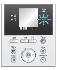
If the **Data Lamp** is flashing, the printer is receiving a print job. Turn off the printer only after printing is finished.
