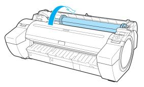
Holding the Roll Holder flange (a), remove the holder from the Roll Holder Slot.
