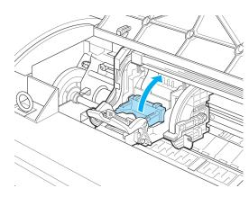
**5** Remove the Printhead and press the **OK** button.
