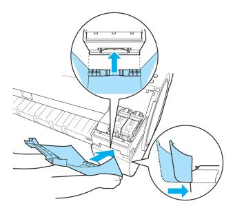
Rotate the Ink Tank Cover and place it on the printer.
