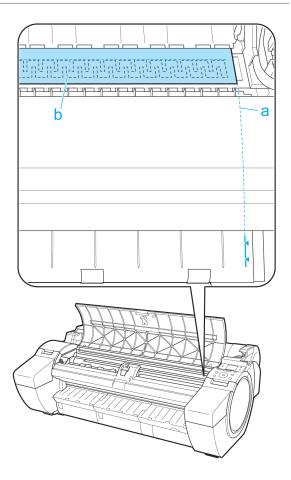
Pull the Release Lever forward and close the Top Cover.
