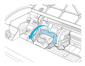
4 Pull up the Printhead Fixer Cover to open it completely.
