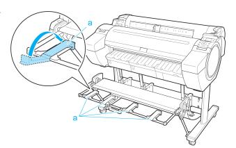
Hold onto the Output stacker handle (a) and pull the Output stacker release lever (b) towards you.
