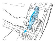
Hold the lnk Tank by the grips and remove it. Press the **OK** button.
