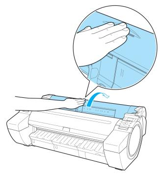
**6** Using both hands, rotate the Roll Holder toward the back to rewind the roll.
