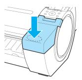
5 Open the Ink Tank Cover and check that it is attached to the printer.
