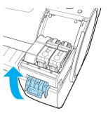
Move the Ink Tank Cover horizontally to align the position with the printer.
