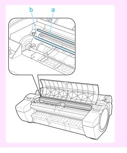
If paper from a roll is jammed by the Paper Feed Slot
