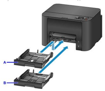
In the upper cassette 1 (A), all sizes of paper compatible with this printer (plain paper, photo paper, envelopes, etc.) can be loaded.
