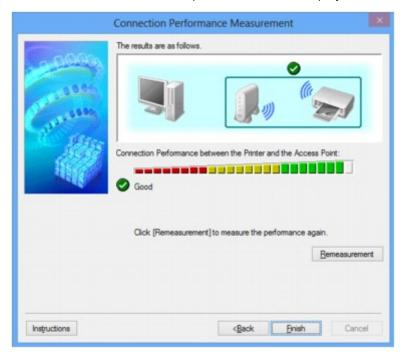
When sis displayed in Connection Performance between the Printer and the Access Point:, the printer can communicate with the access point. Otherwise, refer to displayed comments and the following to improve the status of communication link, and click **Remeasurement**.
