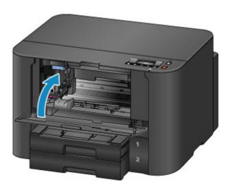
After replacing the ink tanks, the printer starts mixing the ink automatically. Wait until the printer has stopped making operating noise. (This takes about 1 to 2 minutes.)
