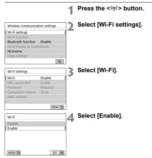
You can also set the Wi-Fi settings with [Wi-Fi settings] under [¥1: Wireless communication settings].
