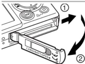
**1** Slide the SD card slot/battery cover in the direction of the arrows.
