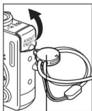
You can use this toggle to open the terminal cover or SD card slot/battery cover.
