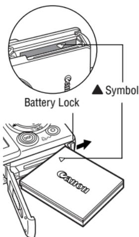
**2** Press the battery lock while inserting the battery pack all the way in until the lock clicks.
