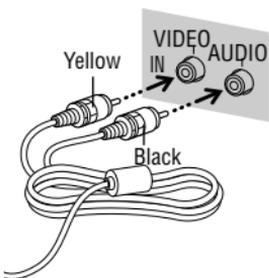
**3** Plug the other ends of the AV cable to the VIDEO IN and AUDIO IN jacks on the TV.
