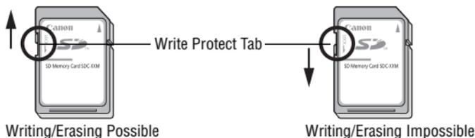
Ensure that the SD card is correctly oriented before inserting it in the camera. It may damage the camera if inserted backward by mistake.
