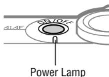
**1 Press the ON/OFF button until the power lamp lights green.**
