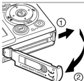
**1** Slide the SD card slot/battery cover in the direction of the arrows.
