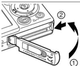
**3** Slide the SD card slot/battery cover closed.
