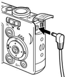
**2** Connect the AV cable to the camera's A/V OUT terminal.
