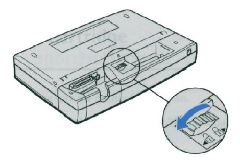
• Disconnect the battery case from the printer..
