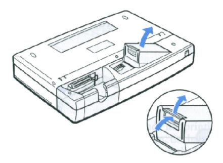
• Lift the battery pack out of the battery compartment.
