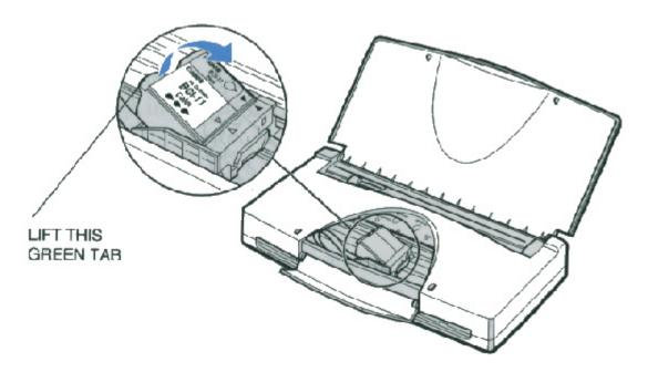
• Make sure you remove both the BJ cartridge and the BJ tank(s).
