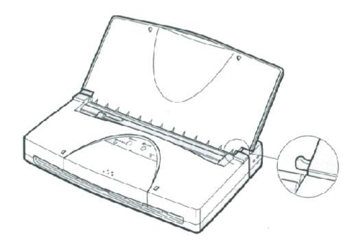
You can now start your print operations. When not printing, close the paper support. When the paper support is open, the battery switch is turned on and the printer is receiving power from the battery pack.
