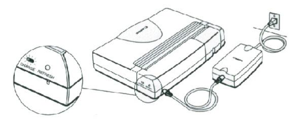
When the battery is fully charged, the CHARGE light turns off.
