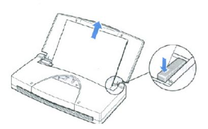
• If the leading edge of the jammed sheet is coming out of the paper exit slot, pull the paper out carefully from the paper exit slot.
