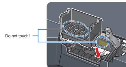
5 Push the Print Head to hold it in place, and lower the Print Head Lock Lever.
