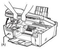
(A) Press the Open button to open the Paper Output Tray if it does not open automatically.
