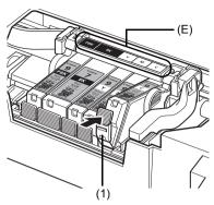
(E) Make sure the position of the tank matches the label.
