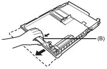
4 Insert the Cassette into the machine. Push the Cassette all the way into the machine.
