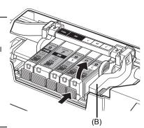
(B) Do NOT touch the Print Head Lock Lever; remove only the ink tank.
