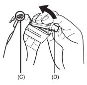
(D) Carefully hold the protective cap when removing it to prevent the ink from staining your fingers. Δ Install the ink tank
