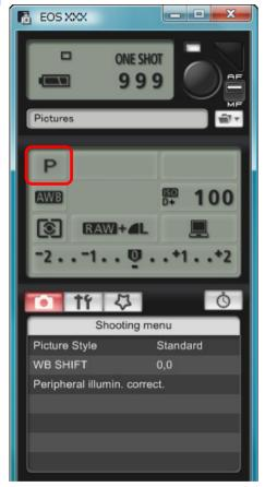
• For cameras other than 1Ds Mk III 1D Mk III 5D Mk III, set the camera's Mode dial to < M > (Manual exposure). Then set the shutter speed to [BULB] in the capture window or on the camera.
