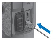
Check the direction of the < • > mark on the plug and push it in.
