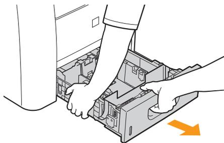
**8** Remove the packing materials with tape.
