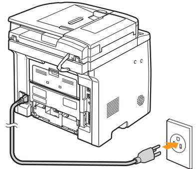
Do not connect the USB cable. Connect the USB cable when installing the software.
