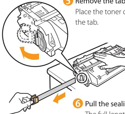
6 Pull the sealing tape completely out.
