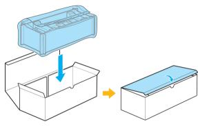
Confirm the Maintenance Cartridge is right-side up, put it in the box, and store it so that it stays level.
