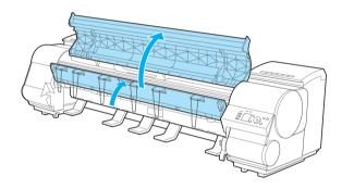
Remove the six Ejection Supports and lower the Ejection Guide.
