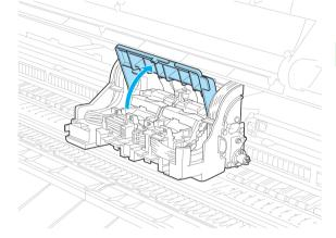
5 Pull the Printhead Fixer Lever forward all the way to open it completely.
