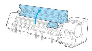
2 If the Cutter Unit or Carriage Cover is dirty, use a damp cloth that you have wrung out completely to wipe it clean.
