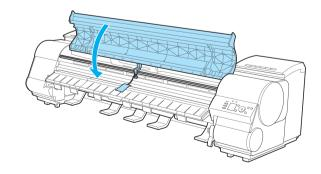
**6** Tape down printer covers to secure them, in the reverse order of tape removal during installation.
