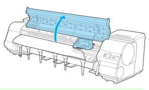
• If the leading edge of the roll jams in the carriage such as when the paper curls strongly, you may be able to avoid paper jamming by setting the roll cutting method to Manual and setting the detection of paper leading edge to [Off].
