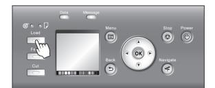
2. Press ▲ or ▼ to select Load Cut Sheet, and then press the OK button.
