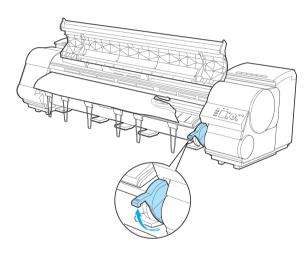
5 Holding the paper on both sides, pull the jammed portion out toward the front. Use scissors or a cutting tool to cut away the printed or wrinkled portion.
