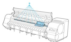
Pull up the Carriage Cover to open it completely.
