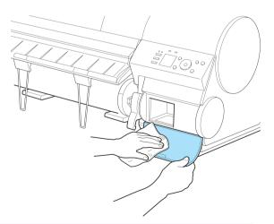
Support the Maintenance Cartridge Cover from underneath as you wipe it.
