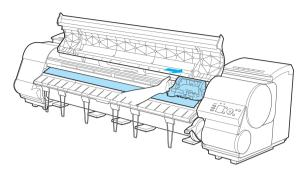
• Always move the Carriage to the right side. If the Carriage is on the left, a Carriage error may occur when you turn on the printer.
