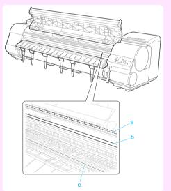
• Never touch the metal contacts of the Carriage. This may damage the printer.
