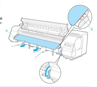
Hold the edge of the roll paper as you gently pull it evenly with both hands to the position of the Ejection Guide (a). Align the right side of the roll paper with the Paper Alignment Line (b), keeping this side parallel to the line, and then lower the Release Lever.
