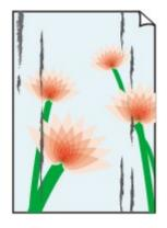
The Edges of Paper Are Smudged Printed Surface Is Smudged
