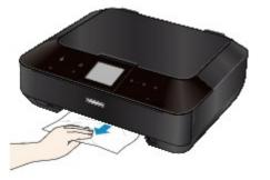
6. If the paper protrudes from the cassette, remove the paper, then reload it after aligning the edges of the sheets.
