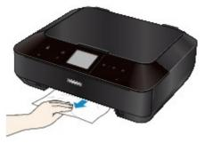
8. If the paper protrudes from the cassette, remove the paper, then reload it after aligning the edges of the sheets.
