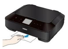
8. If the paper protrudes from the cassette, remove the paper, then reload it after aligning the edges of the sheets.
