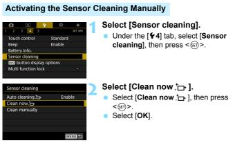
The screen will indicate that the sensor is being cleaned. (A small sound may be heard.) Although there will be a mechanical sound of the shutter during sensor cleaning, the picture will not be recorded to the card.
