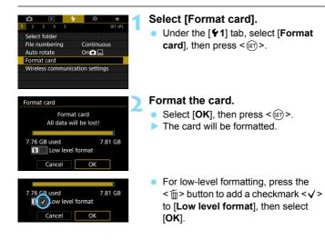
The card capacity displayed on the card format screen may be smaller than the capacity indicated on the card.
