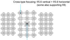
Dual cross-type focusing: f/2.8 right diagonal + f/2.8 left diagonal f/5.6 vertical + f/5.6 horizontal (also supporting f/8)
