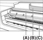
6 Remove the new ink tank from its packaging. Then hold the ink tank as shown and remove the protective cap (A).
