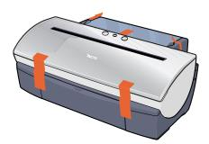
6 Attach protective material to both sides of the printer when packing the printer.
