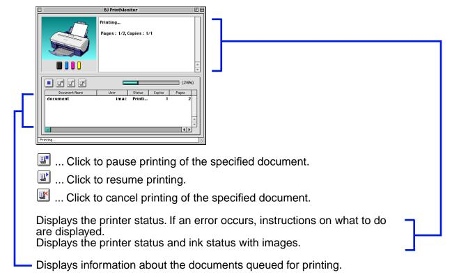
The BJ Print Monitor allows you to change the print order of documents queued for printing. To change the print order, place the mouse pointer over the name of the document, hold the mouse button down while dragging the document name to the new position, then release. Note, however, that you cannot change the print order of a document already printing.
