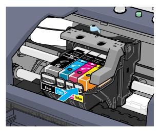
Do not touch the lock lever; remove only the ink tank.
