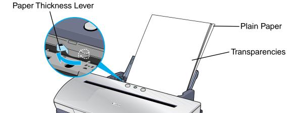
Although you can print on either side of CF-102, best results can be obtained by printing on the side toward which it curls when held by the edge.
