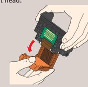
NOTE: Do not touch the print head nozzles and the electrical contacts.
