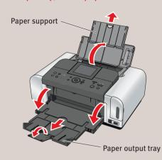
2 Pinch the paper guide and slide it to the left. Load a few sheets of blank paper into the auto sheet feeder, align the paper with the right side of the cover guide, then slide the paper guide toward the left edge of the paper.
