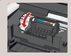
1 Peel back the orange tab completely and remove the plastic wrapper from the Yellow Ink Tank (CLI-8Y).
