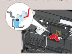
**5** Lower the print head lock lever carefully and press it down.
