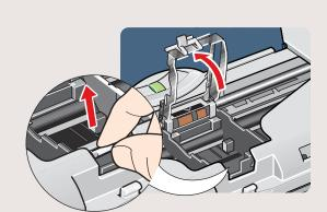
Place the Print Head into the holder by aligning the mark with the mark.
