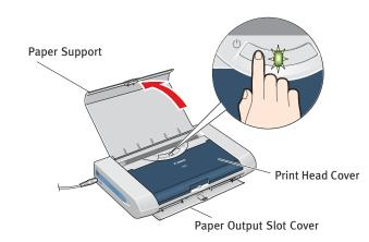
IMPORTANT: Do not open the Print Head Cover before the printer has finished initializing. Wait until the POWER lamp remains fully lit.
