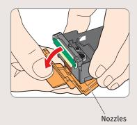
**3** Press in on the Lock Button and raise the gray Lock Lever.
