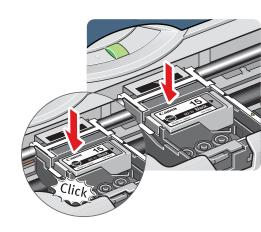
Repeat the procedure for the Color Ink Tank(BCI-16 Color), inserting it into the front slot.
