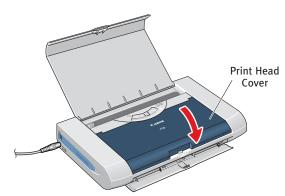
NOTE: The printer will perform a Print Head cleaning after the cover is closed. Wait until the process is complete before proceeding.
