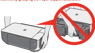
2 Place the machine on a flat and horizontal surface, and do not place any objects in front of the machine.
