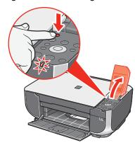
3 Use the ▲ or ▼ button on the Operation Panel to select the language for the LCD, then press the **OK** button.
