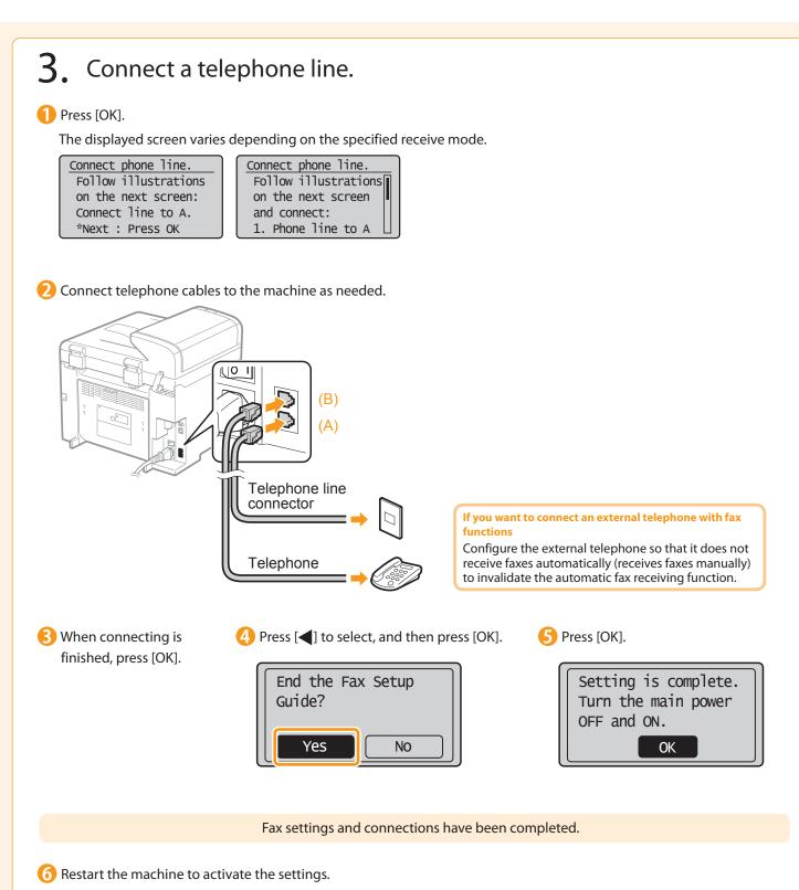
Turn OFF the machine and wait for at least 10 seconds before turning it ON again.
