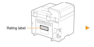
The serial number is located on the rating label centered on the rear side of the machine (a character string of 3 letters and a 5-digit number).
