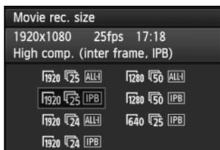
With [**4: Movie rec. size**], you can set the movie's image size, frame rate per second, and compression method. The frame rate switches automatically depending on the [**3: Video system**] setting.
