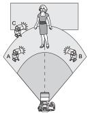
This is a variant of the [¶(A:B)] setup. This setup has group C eliminating the background shadows created by groups A and B
