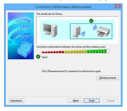
When sis displayed in Connection performance between the printer and the wireless router:, the printer can communicate with the wireless router. Otherwise, refer to displayed comments and the following to improve the status of communication link, and click **Remeasurement**.
