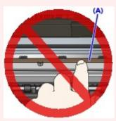
If you soil or scratch the clear film by touching it with paper or your hand, it could damage the machine.
