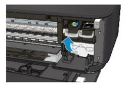
After making sure the FINE cartridge is installed properly, close the paper output cover.
