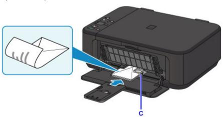
5. Slide the right paper guide (C) to align the paper guides with both sides of the envelopes.
