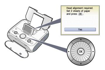
The pattern is printed and the Print Head is aligned automatically.
