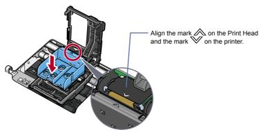
**5** Lower the Print Head Lock Lever carefully by pressing down the tabs on both ends until it clicks into place.
