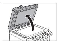
Clean the ADF scanning area (on the left side of the platen glass) and the document feeding roller with a cloth dampened with water. Then wipe the area with a soft, dry cloth.
