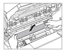
Hold both sides of the jammed paper and gently pull it out upward.
