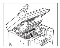
7 Close the printer cover and lower the scanning platform.
