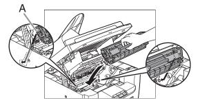
**13** Push down the toner cartridge to make sure it is properly set in the machine.
