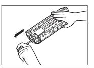
NOTE Do not pull out the seal at an angle.
