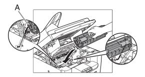
Push the toner cartridge to make sure it is properly set in the machine.
