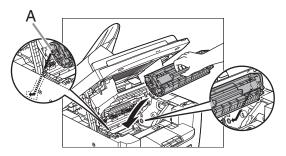
Push the toner cartridge to make sure it is properly set in the machine.
