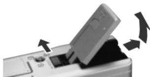
3. Install the battery pack into the battery chamber with the terminals oriented in the direction shown.
