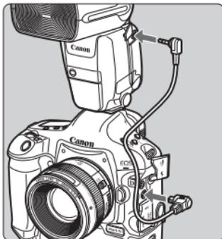
For EOS cameras other than the above that are compatible with E-TTL II/E-TTL autoflash and have an N3 type remote control terminal, the “Release Cable SR-N3” (sold separately) is needed to perform remote release from a slave unit.
