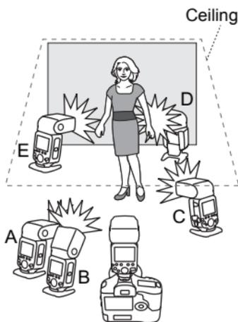
When using an EOS digital camera released since 2012, such as the EOS-1D X, you can shoot with a different flash mode set for each firing group, with up to 5 groups (A/B/C/D/E).
