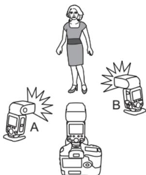
You can divide the slave units into two firing groups, A and B, and adjust the lighting balance (flash ratio) for shooting. The exposure is controlled automatically so that the total flash output of firing groups A and B results in the standard exposure.
