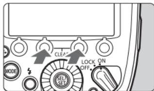
**Press function buttons 2 and 3 simultaneously for 2 seconds or longer.**
