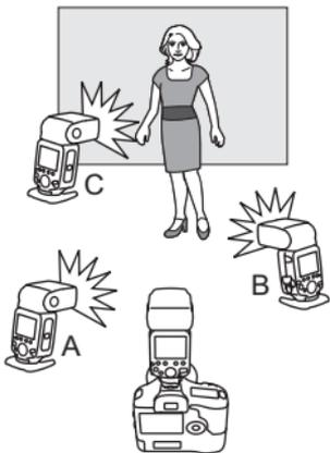
You can add firing group C to firing groups A and B. C is convenient to set lighting so as to eliminate the subject's shadow.
