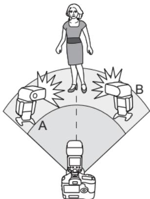
You can divide the slave units into two firing groups, A and B, and adjust the lighting balance (flash ratio) for shooting. The exposure is controlled automatically so that the total flash output of firing groups A and B results in the standard exposure.
