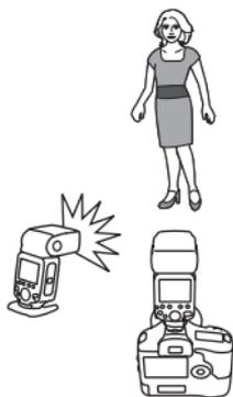
This section describes basic fully automatic wireless shooting when using a 600EX-RT attached to the camera (master) and a 600EX-RT wirelessly controlled (slave).
