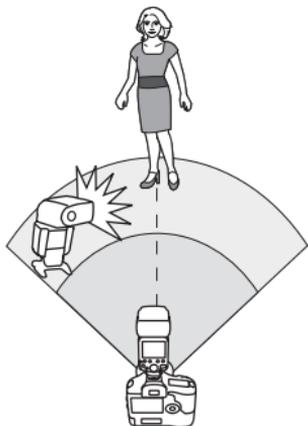
This section describes basic fully automatic wireless shooting when using a 600EX-RT/600EX attached to the camera (master) and a 600EX-RT/600EX wirelessly controlled (slave).
