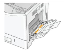
Gently load paper with the printing side face-down under the load limit guides (A) until it touches the back of the tray.
