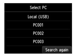
Tap **Local (USB)** for a USB-connected computer, or tap the computer to forward the scanned data for a network-connected computer.
