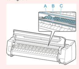
3. If ventilation duct (A) is dirty, use damp cloth that you have wrung out completely to wipe it clean.
