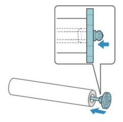
3. Load roll paper in printer or roll unit. (See "Loading the Upper Roll on the Printer.") (See "Loading the Lower Roll on the Roll Unit.")
