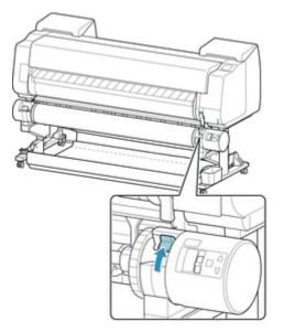
9. Hold roll holder by its flanges (A), and remove from roll unit.
