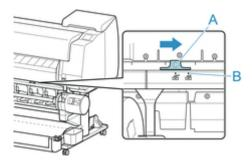
10. Change **Inward/Outward Winding Changeover** switch on roll unit to desired winding direction.
