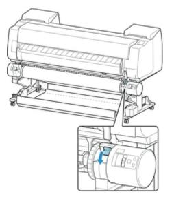
7. Change feed flap switch on top of roll unit to feed icon position on the left.
