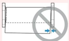
Depending on the paper, the roll paper may be scratched when being fed and not feed well. In this case, you must feed the paper manually after setting Paper retention setting to Release on the touch screen. Lift the release lever, advance the roll paper until its leading edge appears on platen, lower the release lever, and then proceed to the next step. However, if Paper retention setting is set to Release, automatic switching of the upper and lower rolls is not possible.
