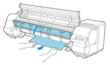
After removing the paper, inspect the interior to ensure paper fragments or other objects do not remain, and lower the output guide.
