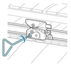
4. Remove cutter blade while holding A.
