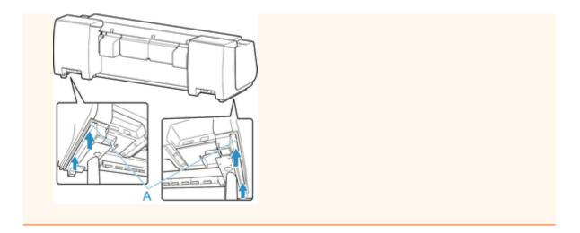
2. Remove tape and packaging material attached to the printer. Also open the top cover and remove stoppers and spacers inside the printer.
