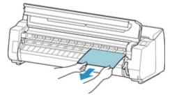
6. If you cannot see the paper, lift the output guide, remove the roll holder, and remove the jammed paper from underneath.
