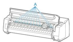
4. While pressing button (A) in center of print head lock lever, pull it forward to open it until it stops.
