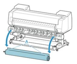
10. Push holder stopper lever (A) toward shaft to release lock, and while holding in position (B), remove holder stopper from roll holder.
