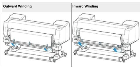
4. While making sure that roll paper is flat, secure left edge of roll paper to paper core with tape.
