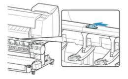
8. Pull out roll paper evenly, insert leading edge between roll paper and arrows (A) directly beneath it, and feed roll paper until you hear a sound.
