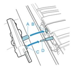
6. Install while aligning fixing part included with replacement cutter blade with center of cutter blade.
