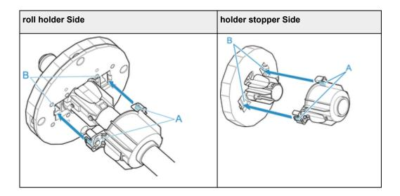
4. Insert paper core, which is for winding roll paper, into roll holder.
