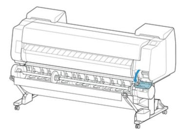
3. Hold the used maintenance cartridge by the grip (A) with one hand and put your other hand under the maintenance cartridge to hold it firmly on the bottom, keeping it level as you pull it out.
