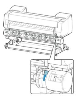
5. Hold flanges (A) so that roll holder's white gear is on left, align roll holder shaft with roll holder slot left and right guide grooves (B), and load.
