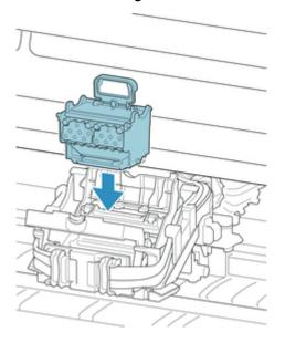
11. Lower print head locking cover to front and lock print head.
