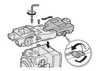
You can use the optional RD-1 Rod Clamp to use the camera with a commercially available viewfinder or other accessories with a Ø 15 mm (0.59 in.) rod.
