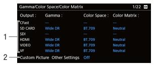
1 Gamma curve, color space and color matrix used for recordings, video output and displays [CFast]: Settings used for clips recorded on the CFast card (☐ 123, 126) [SD CARD]: Settings/LUT used for clips recorded on the SD card (☐ 110) [SDI], [HDMI]: Settings/LUT used for video output from the respective terminals (☐ 144)
