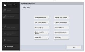
Press the [Device Configuration] - [ScanFront Maintenance] - [Roller counter reset] button to display the roller counter reset screen.
