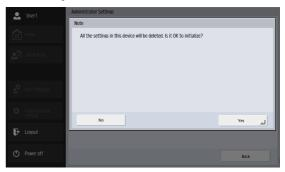
3. Confirm the message and press [Yes] to perform initialization, and the scanner will turn OFF.
