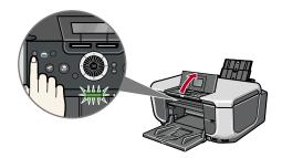
**5** Use the  $\blacktriangle$  or  $\checkmark$  button on the Operation Panel to select the language for the LCD, then press the **OK** button.
