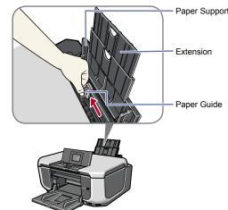
2 Load two sheets of supplied paper (MP-101) into the Auto Sheet Feeder with the printing side (whiter side) facing up, align the paper with the right side of the Cover Guide, then slide the Paper Guide against the paper stack.
