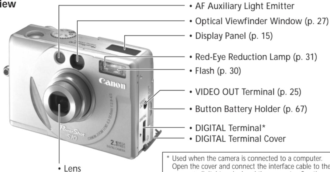
\* Used when the camera is connected to a computer. Open the cover and connect the interface cable to the camera's digital terminal and the computer. See the *Software Starter Guide* for additional information.
