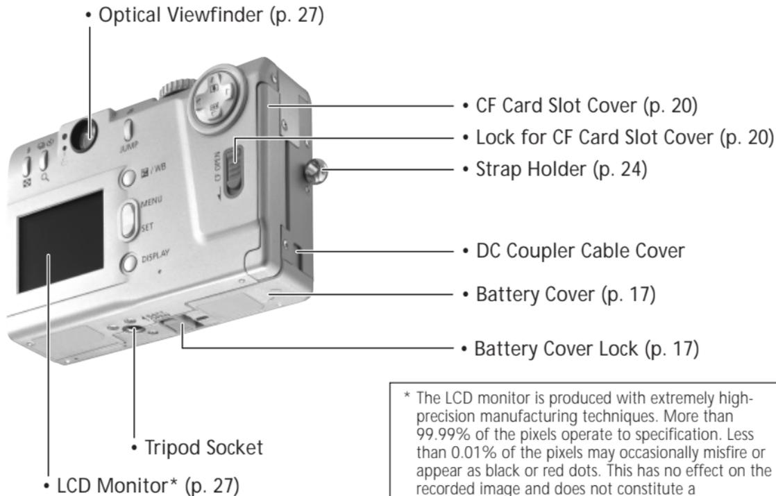
\* The LCD monitor is produced with extremely high-precision manufacturing techniques. More than 99.99% of the pixels operate to specification. Less than 0.01% of the pixels may occasionally misfire or appear as black or red dots. This has no effect on the recorded image and does not constitute a malfunction.
