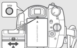
Adjust the viewfinder as necessary with the dioptic adjustment lever. You can also change the brightness of the screen (□ 27). Using the bright setting will shorten the effective usage time of the battery pack.
