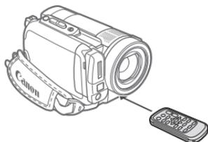
Point the wireless controller at the camcorder's remote sensor when you press the buttons.
