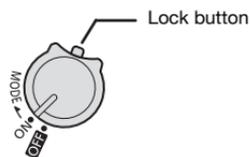
In addition to turning the camcorder on and off, the **POWER** switch also toggles the camcorder's operating mode.
