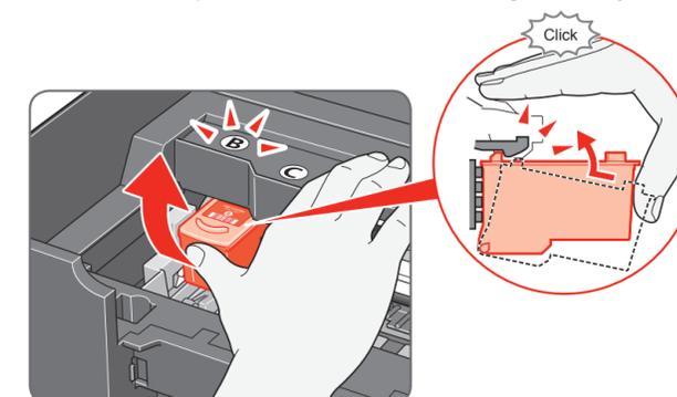
**5** Repeat the procedure for the Color FINE Cartridge, inserting it into the right slot **C**.
