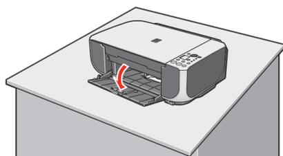
**2** Lift the Scanning Unit (Printer Cover), and pull the Scanning Unit Support down into place.
