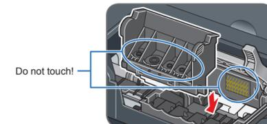
5 Push the Print Head to hold it in place, and lower the Print Head Lock Lever carefully.
