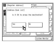
To cancel erasing, press [No]. The message <Erased.> appears for approximately two seconds on the touch panel display. Press [Done] repeatedly until the Send Basic Features screen appears.
