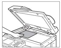
The surface of the original that you want to scan must be placed face down.
