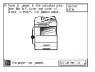
Press the button on the left cover of the main unit, and open the left cover.
