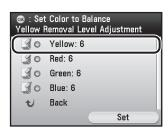
Use [◀], [▶] or ⊚ (Scroll Wheel) to adjust the strength of the color, then press [OK].
