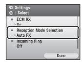
Use  $[\nabla]$ ,  $[\triangle]$  or o (Scroll Wheel) to select the desired receive mode, then press [OK].
