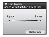
Move the indicator to the left to make the exposure lighter or move it to the right to make the exposure darker.
