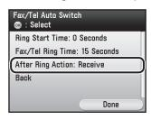
⑦ Use [▼], [▲] or ⊚ (Scroll Wheel) to select the action the machine will take after the ringing ends, then press [OK].
