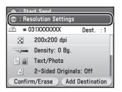
5 Use  $[\nabla]$ ,  $[\triangle]$  or 0 (Scroll Wheel) to select the desired resolution, then press [OK].
