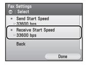
Use [▼], [▲] or ⊚ (Scroll Wheel) to select the desired start speed, then press [OK].
