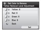
③ Use  $[\P]$ , [A], [A], [P] or ⑥ (Scroll Wheel) to adjust the strength of the color, then press [OK].
