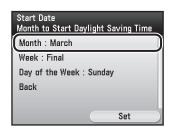
Use [▼], [▲] or ⑥ (Scroll Wheel) to select the month when the daylight saving time starts, then press [OK].
