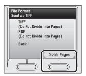
If you want to separate multiple images and send them as separate files, each of which consists of only one page, use [▼], [▲] or ⑥ (Scroll Wheel) to select <On>, then press [OK] twice.
