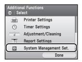
If the System Manager ID and System Password have been set, enter the System Manager ID and System Password using ①-③ (numeric keys), then press ⑩ (Log In/Out).
