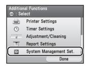
If the System Manager ID and System Password have been set, enter the System Manager ID and System Password using ① – ⑨ (numeric keys), then press ⑩ (Log In/Out).
