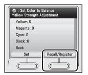
Use [▼], [▲] or ⊚ (Scroll Wheel) to select the memory key that you want to store the color balance setting under, then press the right Any key to select <Register/Erase>.
