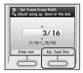
② Use [▼], [▲] or ⊚ (Scroll Wheel) to select the desired frame erase borders, then press [OK].
