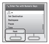
Enter the number of the fax information service using  $\bigcirc$   $\bigcirc$   $\bigcirc$   $\bigcirc$  (numeric keys).
