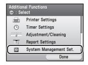
If the System Manager ID and System Password have been set, enter the System Manager ID and System Password using ③ – ⑨ (numeric keys), then press ⑩ (Log In/Out).
