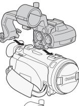
2 Firmly tighten the front and rear screws with a coin or similar object.
