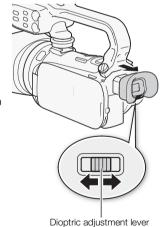
If you wear glasses, you may find the viewfinder easier to use if you flip back the outer edge of the eye cup toward the camcorder body by pushing the points indicated by the arrows in the illustration.
