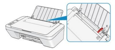
If there are any foreign objects in the rear tray, be sure to turn off the machine, unplug it from the power supply, then remove the foreign object.
