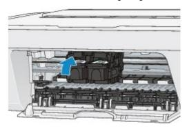
After confirming that the FINE cartridge is installed properly, close the cover.
