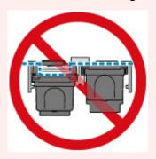
The machine cannot print unless both the color FINE cartridge and black FINE cartridge are installed. Be sure to install both cartridges.
