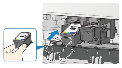
• Insert the FINE cartridge gently so that it does not hit the electrical contacts on the FINE cartridge holder.
