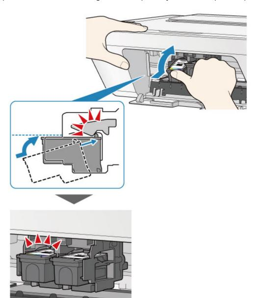
Check if the FINE cartridge is installed correctly.
