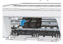
After confirming that the FINE cartridge is installed properly, close the cover.
