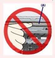
If the paper or your hands touch the clear film and blot or scratch it, the machine can be damaged.
