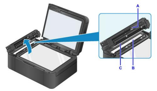
Make sure not to leave any residue, especially on the glass surface.
