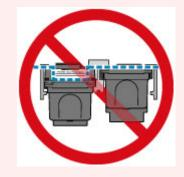
• The machine cannot print unless both the color FINE cartridge and black FINE cartridge are installed. Be sure to install both cartridges.
