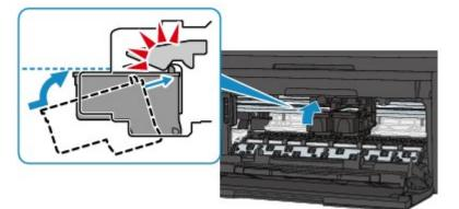
When the FINE cartridge is installed properly, you hear an electric sound once.
