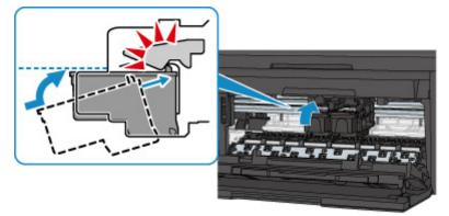
When the FINE cartridge is installed properly, you hear an electric sound once.
