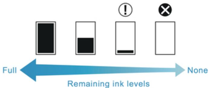
If the touch screen indicates to replace the ink tank, replace the ink tank. If a message is displayed indicating to check the remaining ink levels, or after tasks that consume a lot of ink such as large-format printing or head cleaning, check the remaining levels and replace ink tank as needed.
