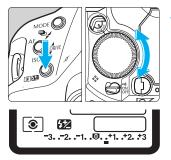
While pressing the < ᠍₺ > button, turn the < > dial to set the desired flash exposure compensation amount.
