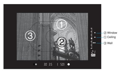
• While referring to the exposure level indicator's three spot metering marks, you can set exposure compensation to obtain the desired result.
