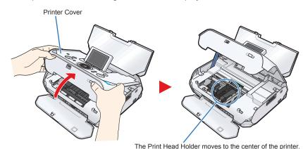
If the Printer Cover is left open for more than 10 minutes, the Print Head Holder moves to the right. Close and reopen the Printer Cover to return the holder to
