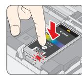
nost) part of the ink tank (A) is sticking up, push down on the Canon logo on the ink tank as illustrated below. Do not remove the ink tank
